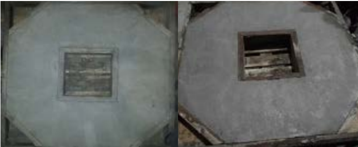
Fig. 2: Horizontal shotcrete test panels before abrasion test (control - left. Hard Cem - right.)
