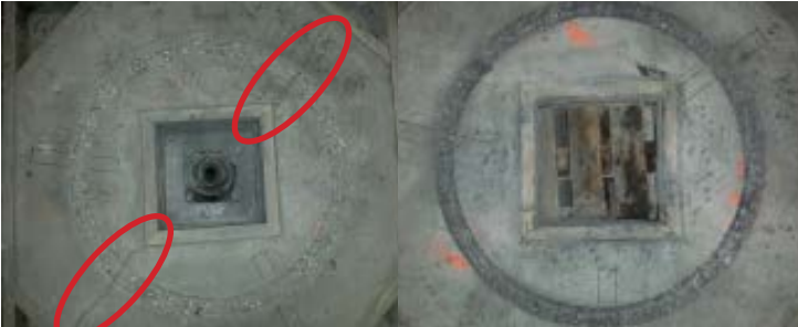
Fig. 3: Horizontal shotcrete test panels after abrasion test (control - left. Hard Cem - right.) Control cracks highlighted in red. No Hard-Cem cracks developed during the test.
