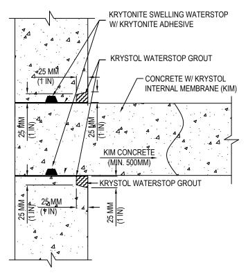
WALL TO ELEVATED SLAB DOUBLE PROTECTION
