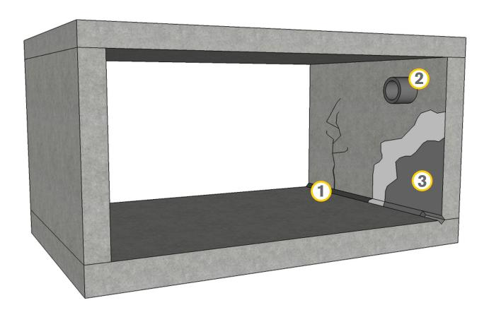
Negative side waterproofing for below grade structures where there has been no waterproofing or the waterproofing membrane has failed.
