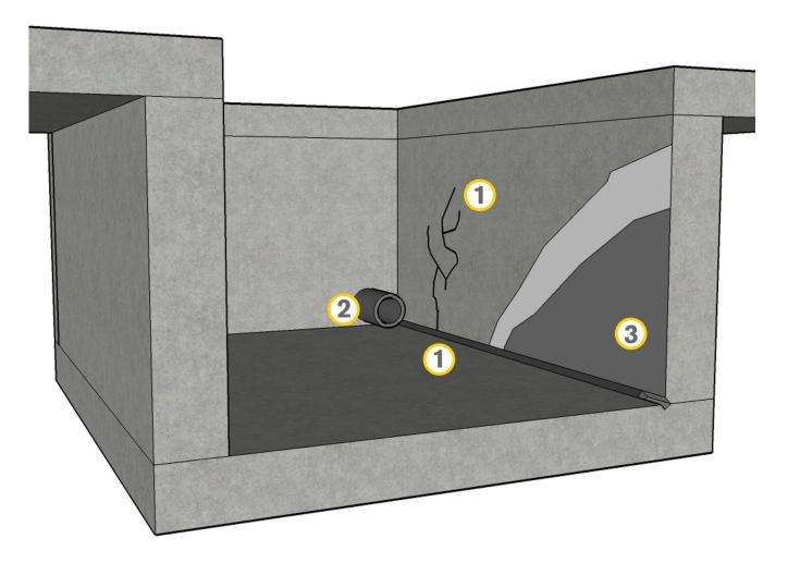
Negative side waterproofing for below grade structures where there has been no waterproofing or the waterproofing membrane has failed.
