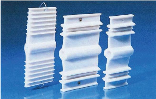
PVC waterstops are flat strips of high-quality PVC that are embedded into both sides of a construction joint to provide a physical barrier. Specially shaped to create a better bond with concrete, PVC waterstops are available in a variety of thicknesses, widths and sizes.
