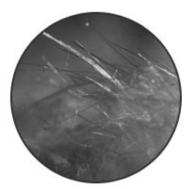
Krystol is a mixture of cement organic waterproofing ingredients that work as a catalyst to further react unhydrated cement particles and promote the hydration process growing more and longer crystals that penetrate deeply into the pores and capillaries of concrete. rendering waterproof - permanently.
