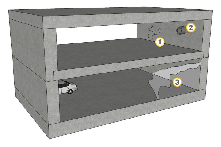
Negative side waterproofing for below grade structures where there has been no waterproofing or the waterproofing membrane has failed.
