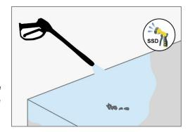
**NOTE:** Acid etching is not recommended. If acid etching used, all traces of acid must neutralized and rinsed away before applying the Krystol T1.
