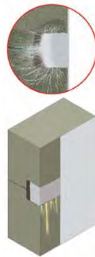
Step 4: Apply Krystol T1 to the surface.
